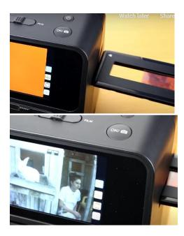
6. To switch from negatives to slides or vice versa, press the center button (home), and select the desired option.
