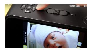
10. To adjust the color of the image, press the right arrow on the scanner, then the top button or "play" icon, then arrow left/right to change red coloring of image.
