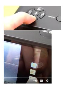
To adjust the color and brightness of the image, press the right arrow on the scanner. Arrow left or right to darken/lighten. Click OK to save settings. This will affect all FUTURE images scanned.
