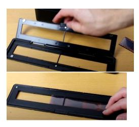
5. Load the left side of the holder into the right side of the scanner. Slide inside until you can see an image on the LCD screen. Press OK to scan. This image is now saved to the inserted SD card. Repeat until all images are scanned. Slide the holder out and unload/load more negatives for scanning.
